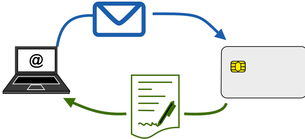
Figure 6.1: Client based signing: The message is transferred to the SmartCard and the generated Signature is returned
