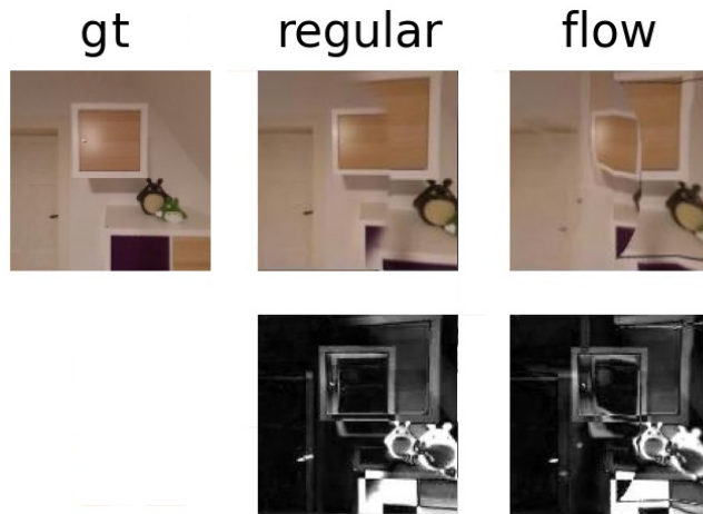
Figure 4.43.: Right face of viewpoint D (high values for both regular and flow-based blending): The high error values are due to the proximity to the cabinet, which is not reprojected correctly in the regular blending, and for which the optical flow algorithms also seems to have failed.
