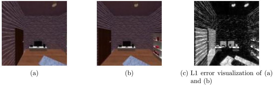
Figure 4.2.: Example visualization of L1 RGB error. The error values are oversaturated, which makes them more visible.
