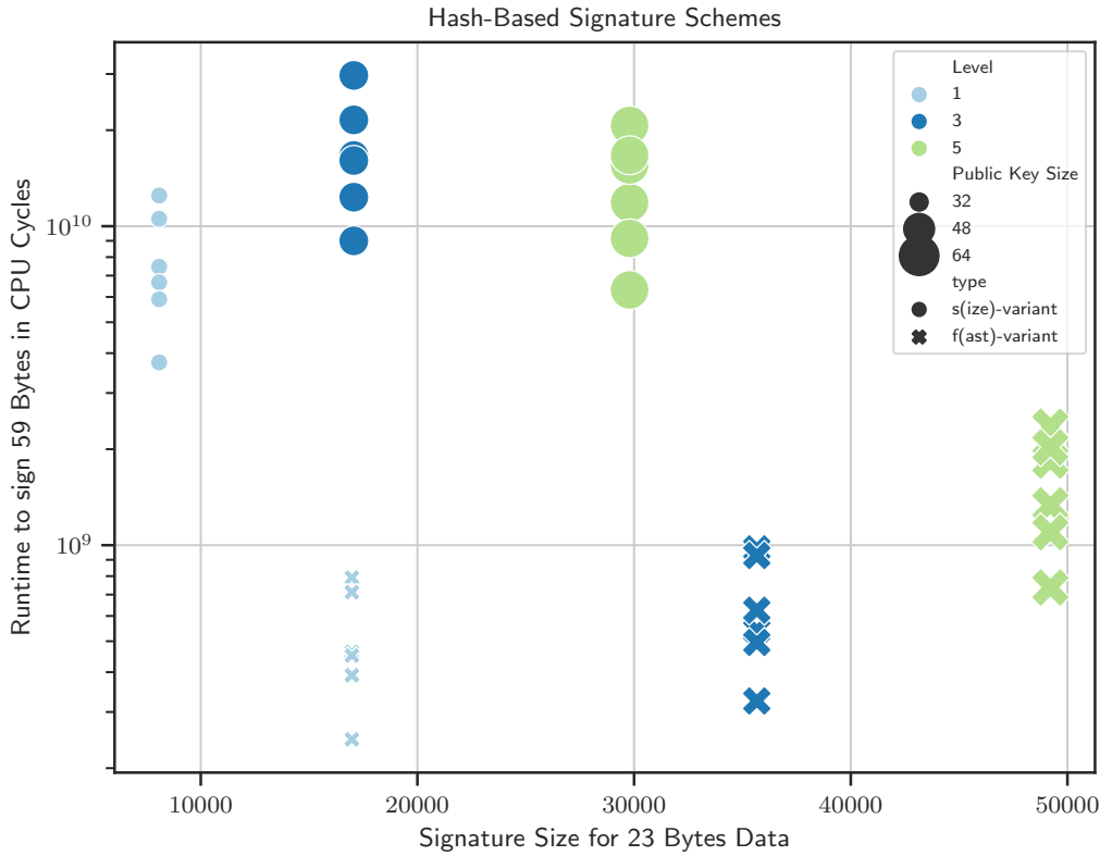
Figure 2.10: Overview of the current implementation of hash-based signature schemes in Round 3 of the NIST PQ standardization project. All security level 3 implementations are shown. The y-axis shows the latency to sign a 59 Byte message in CPU cycles on a logarithmic axis. The x-axis shows the size of a signature for a 23 Byte message. Benchmark results are part of eBACS[Be]
