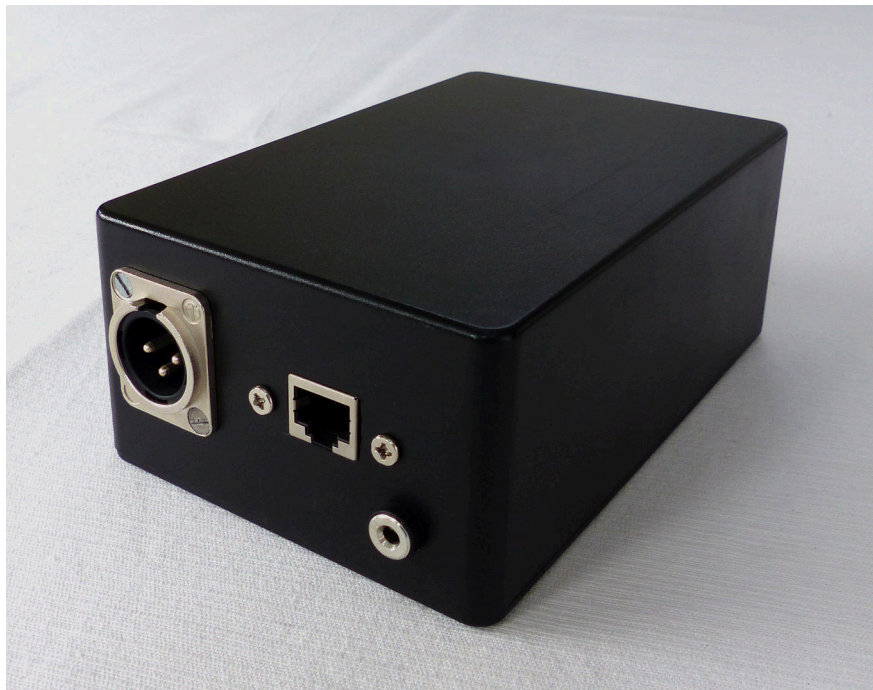
Figure 4.13: Finished PC-DMX interface.
