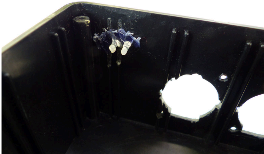
Figure 4.11: Optical waveguides for indicator LEDs.
