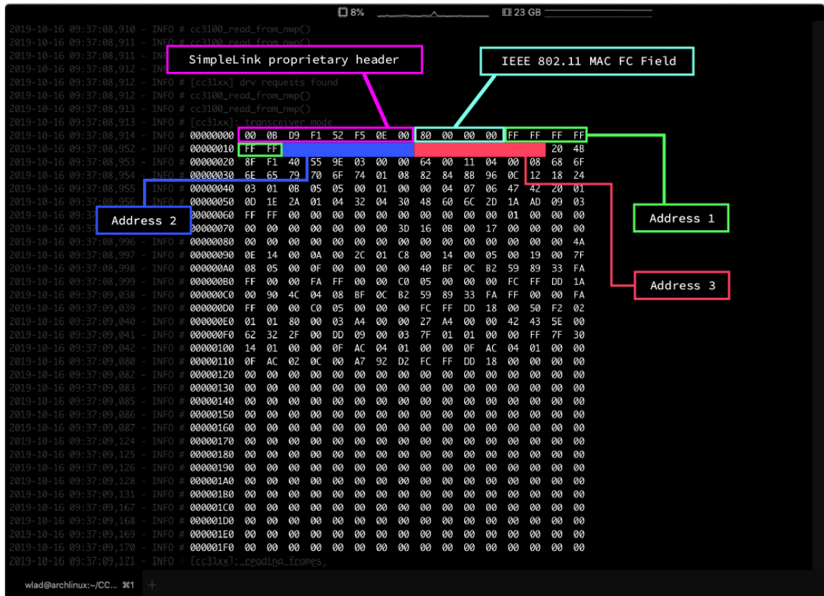
Figure 5.1: Example NWP socket frame received via the CC31xx driver. Sensitive MAC addresses were redacted
