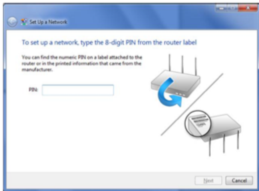
Figure 6: Windows Connect Now Wizard acting as a Registrar (Windows 7)
